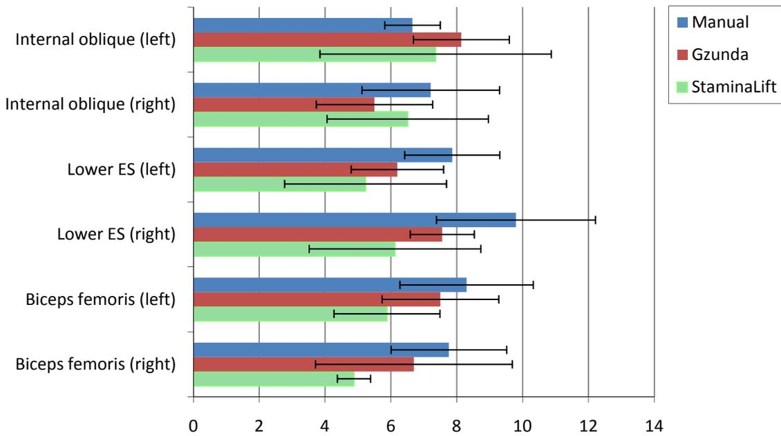
Figure 11: %MVC for the left and right internal oblique, lower ES and biceps femoris. The mean and standard deviation is shown for each measurement
